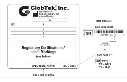
A=ICT / ITE / Medical Power Supply/Class 2/Household Power Supply B=P/N: (料号) TR9CI2700LCPCIMR6B C=Model (型号) GTM96600-6524-T3 D=Input (输入)100-240V~, 50-60Hz, 1.5A E=Output (输出)24.0 V === 2.7 A, 65.00W
