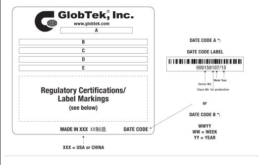
A=ICT/ITE Power Supply B=P/N: (料号) TR9CI2700LCP-N(R6B) C=Model (型号) GT-46600-6524-T3 D=Input (输入)100-240V~, 50-60 Hz, 1.5A E=Output (输出)24.0 V === 2.7 A, 65.00W
