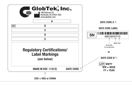
A=ICT / ITE / Medical Power Supply/Class 2/Household Power Supply B=P/N: (料号) TR9CI2500T00CIMR6B C=Model (型号) GTM96600-6024-T3 D=Input (输入)100-240V~, 50-60Hz, 1.5A E=Output (输出)24.0 V === 2.5 A, 60.00W
