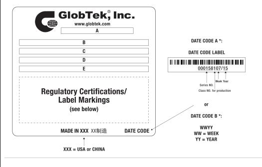
A=ICT/ITE Power Supply B=P/N: (料号) TR9CI2500LCP-N(R6B) C=Model (型号) GT-46600-6024-T3 D=Input (输入)100-240V~, 50-60 Hz, 1.5A E=Output (输出)24.0 V === 2.5 A, 60.00W
