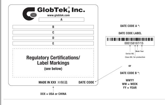
A=ICT/ITE Power Supply B=P/N: (料号) TR9CI1670LCP-N(R6B) C=Model (型号) GT-46400-4024-T3 D=Input (输入)100-240V~, 50-60 Hz, 1.0A E=Output (输出)24.0 V == 1.66 A, 40.00W
