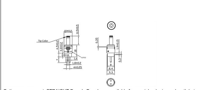
Option upon request: STRAIGHT Female Barrels are available for special order in any length between 9mm-14mm
