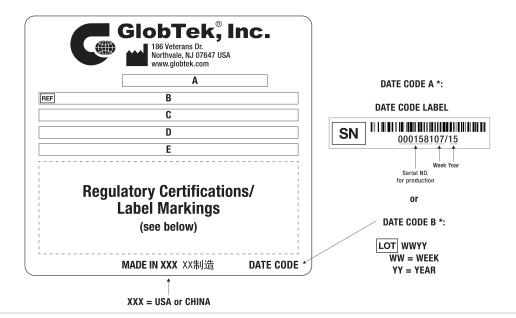
A=Medical/ICT/ITE/Household use Power Supply B=P/N: (料号) TR9CI1500LCPIMR6B C=Model (型号) GTM96300-3624-T3 D=Input (输入)100-240V~, 50-60 Hz, 1.0A E=Output (输出)24.0 V == 1.5 A, 36.00W
