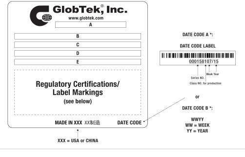
A=Medical/ICT/ITE/Household use Power Supply B=P/N: (料号) TR9CH9440LCPIMR6B C=Model (型号) GTM961800P17018-T3 D=Input (输入)100-240V~, 50-60Hz, 2.2A E=Output (输出)18.0 V === 9.44 A, 170.00W
