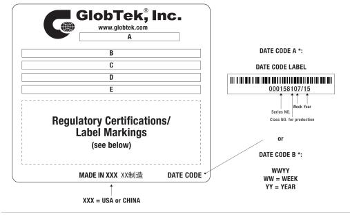
A=Medical/ICT/ITE/Household use Power Supply B=P/N: (料号) TR9CH9440CCPIMR6B C=Model (型号) GTM961800P17018-T3 D=Input (输入)100-240V~, 50-60Hz, 2.2A E=Output (输出)18.0 V === 9.44 A, 170.00W
