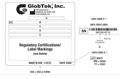
A=Medical/ICT/ITE/Household use Power Supply B=P/N: (料号) TR9CH8330CCPCIMR6B C=Model (型号) GTM961600P15018-T3 D=Input (输入)100-240V~, 50-60 Hz, 2.2A E=Output (输出)18.0 V === 8.33 A, 150.00W
