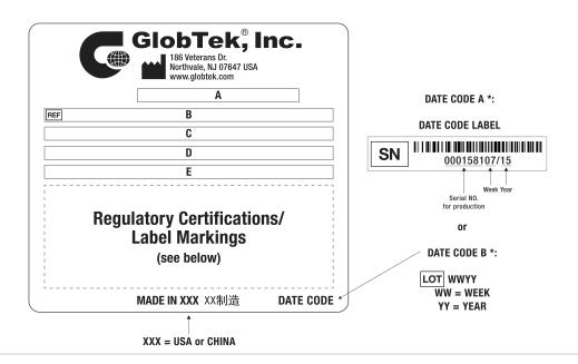
A=ICT / ITE / Medical Power Supply B=P/N: (料号) TR9CH6666T00-IM(R6B) C=Model (型号) GTM961200P12018-T3 D=Input (输入)100-240V~, 50-60 Hz, 1.5 A E=Output (输出)18.0 V == 6.66 A, 120.00W
