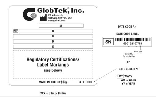
A=ICT / ITE / Medical Power Supply/Class 2/Household Power Supply B=P/N: (料号) TR9CH3610T00IMCFR6B C=Model (型号) GTM96600-6518-T3-CF D=Input (输入)100-240V~, 50-60Hz, 1.5A E=Output (输出)18.0 V === 3.61 A, 65.00W
