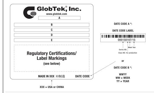
A=ICT / ITE / Medical Power Supply/Class 2/Household Power Supply B=P/N: (料号) TR9CH3610T00CIMR6B C=Model (型号) GTM96600-6518-T3 D=Input (输入)100-240V~, 50-60Hz, 1.5A E=Output (输出)18.0 V === 3.611 A, 65.00W
