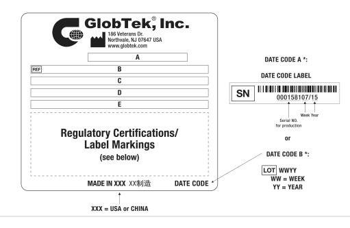
A=ICT / ITE / Medical Power Supply/Class 2/Household Power Supply B=P/N: (料号) TR9CH1000T00-IMR6B C=Model (型号) GTM96180-1830-12.0-T3 D=Input (输入)100-240V~, 50-60 Hz, 0.6 A E=Output (输出)18.0 V === 1.0 A, 18.00W
