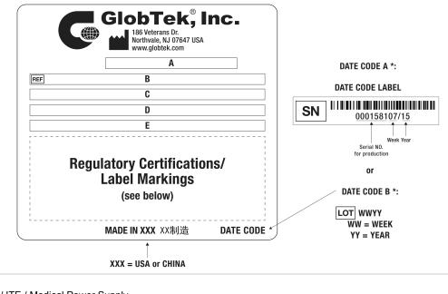
A=ICT / ITE / Medical Power Supply B=P/N: (料号) TR9CG8000LCP-IM(R6B) C=Model (型号) GTM961200P12015-T3 D=Input (输入)100-240V~, 50-60 Hz, 1.5 A E=Output (输出)15.0 V === 8.0 A, 120.00W
