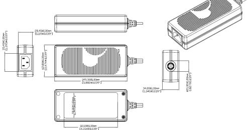
Alternative housing with input cord clamp to prevent accidental removal of the power cord. Product PN# ends with suffix "CL"
