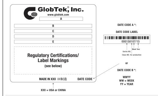
A=ICT / ITE / Medical Power Supply/Class 2/Household Power Supply B=P/N: (料号) TR9CG6000T00-IM(R6B) C=Model (型号) GTM96900P9015-T3 D=Input (输入)100-240V~, 50-60Hz, 1.5A E=Output (输出)15.0 V === 6.0 A, 90.00W
