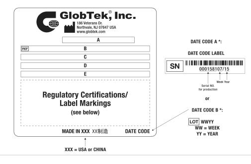
A=ICT / ITE / Medical Power Supply/Class 2/Household Power Supply B=P/N: (料号) TR9CG4330T00CIMR6B C=Model (型号) GTM96600-6515-T3 D=Input (输入)100-240V~, 50-60Hz, 1.5A E=Output (输出)15.0 V ---- 4.33 A, 65.00W
