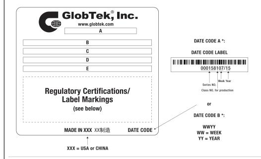
A=ICT / ITE / Medical Power Supply/Class 2/Household Power Supply B=P/N: (料号) TR9CG4000T00CIMR6B C=Model (型号) GTM96600-6015-T3 D=Input (输入)100-240V~, 50-60Hz, 1.5A E=Output (输出)15.0 V == 4.0 A, 60.00W
