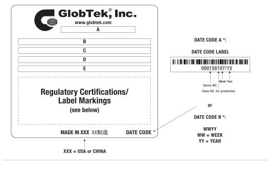
A=ICT/ITE Power Supply B=P/N: (料号) TR9CG2660CCP-N(R6B) C=Model (型号) GT-46400-4015-T3 D=Input (输入)100-240V~, 50-60 Hz, 1.0A E=Output (输出)15.0 V == 2.66 A, 40.00W
