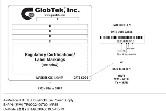
D=Input (输入)100-240V~, 50-60 Hz, 1.0A E=Output (输出)15.0 V === 2.4 A, 36.00W
