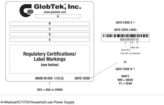
A=Medica//C1/1E/Housenoid use Power Supp B=P/N: (料号) TR9CG2400LCPCIMR6B C=Model (型号) GTM96300-3619.5-4.5-T3 D=Input (输入)100-240V~, 50-60 Hz, 1.0A E=Output (输出)15.0 V === 2.4 A, 36.00W
