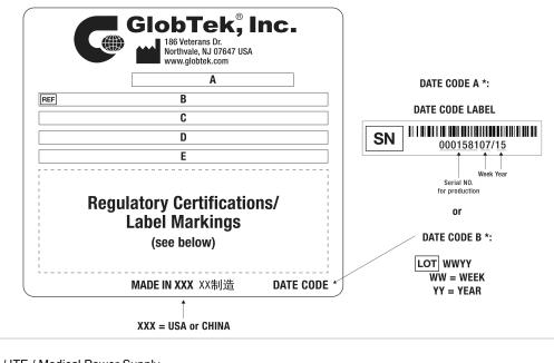
A=ICT / ITE / Medical Power Supply B=P/N: (料号) TR9CE9200YL4CIM(R6B) C=Model (型号) GTM961200P11012-T3 D=Input (输入)100-240V~, 50-60 Hz, 1.5 A E=Output (输出)12.0 V === 9.2 A, 110.40W
