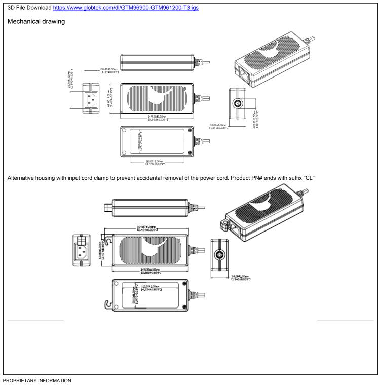
PROPRIETARY INFORVIATION PROPRIETARY OF GLOBTEK, INC. ANY REPRODUCTION, DISCLOSURE OR USE OF THIS DRAWING, IN WHOLE OR IN PART, IS HEREBY PROHIBITED EXCEPT AS SPECIFIED IN WRITING BY GLOBTEK, INC. © GlobTek, Inc. 2018 - 2025 guest / 05/14/2025 11:41:11 AM GMT CLONED FROM TR9CI6666MF6CIMR6B
