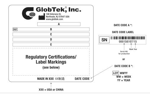
A=ICT / ITE / Medical Power Supply/Class 2/Household Power Supply B=P/N: (料号) TR9CE7500FILRPNIMR6B C=Model (型号) GTM96900P9012-T3 D=Input (输入)100-240V~, 50-60Hz, 1.5A E=Output (输出)12.0 V === 7.5 A, 90.00W
