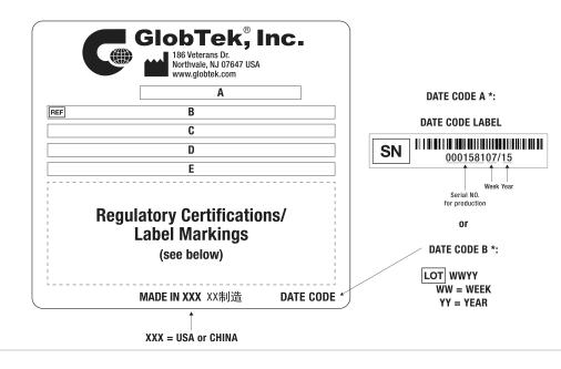
A=ICT / ITE / Medical Power Supply/Class 2/Household Power Supply B=P/N: (料号) TR9CE7080LPCIMR6BLPS C=Model (型号) GTM96900P8512-T3Z D=Input (输入)100-240V~, 50-60Hz, 1.5A E=Output (输出)12.0 V === 7.08 A, 85.00W
