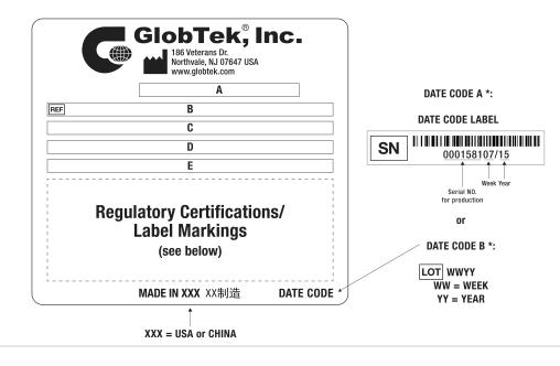
A=ICT / ITE / Medical Power Supply/Class 2/Household Power Supply B=P/N: (料号) TR9CE5410T00CIMR6B C=Model (型号) GTM96600-6512-T3 D=Input (输入)100-240V~, 50-60Hz, 1.5A E=Output (输出)12.0 V === 5.41 A, 65.00W
