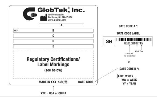
A=ICT / ITE / Medical Power Supply/Class 2/Household Power Supply B=P/N: (料号) TR9CE5410LCPCIMR6B C=Model (型号) GTM96600-6512-T3 D=Input (输入)100-240V~, 50-60Hz, 1.5A E=Output (输出)12.0 V === 5.41 A, 65.00W
