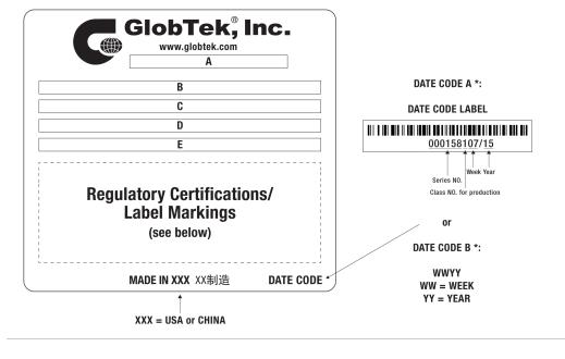
A=ICT/ITE Power Supply B=P/N: (料号) TR9CE5000CCP-N(R6B) C=Model (型号) GT-46600-6012-T3 D=Input (输入)100-240V~, 50-60 Hz, 1.5A E=Output (输出)12.0 V === 5.0 A, 60.00W
