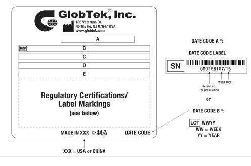
A=Medical/ICT/ITE/Household use Power Supply B=P/N: (料号) TR9CE3000CLWCIMR6B C=Model (型号) GTM96300-3614.5-2.5-T3 D=Input (输入)100-240V~, 50-60 Hz, 1.0A E=Output (输出)12.0 V === 3.0 A, 36.00W
