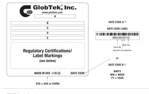
A=ICT/ITE Power Supply B=P/N: (料号) TR9CE1500LCP-N(R6B) C=Model (型号) GT-46181-1812-T3 D=Input (输入)100-240V~, 50-60 Hz, 0.5A E=Output (输出)12.0 V == 1.5 A, 18.00W
