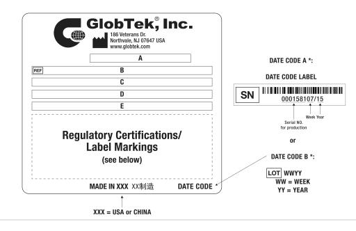
A=ICT / ITE / Medical Power Supply/Class 2/Household Power Supply B=P/N: (料号) TR9CE1500CCP-IMR6B C=Model (型号) GTM96180-1817.9-5.9-T3 D=Input (输入)100-240V~, 50-60 Hz, 0.6 A E=Output (输出)12.0 V === 1.5 A, 18.00W
