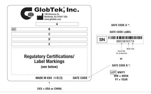
A=Medical/ICT/ITE/Household use Power Supply B=P/N: (料号) TR9CD3333T00IMR6B C=Model (型号) GTM96300-3010.5-1.5-T3 D=Input (输入)100-240V~, 50-60 Hz, 1.0A E=Output (输出)9.0 V === 3.33 A, 30.00W
