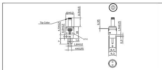
Option upon request: STRAIGHT Female Barrels are available for special order in any length between 9mm-14mm
