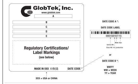
A=ICT / ITE / Medical Power Supply/Class 2/Household Power Supply B=P/N: (料号) TR9CC2400T00-IMR6B C=Model (型号) GTM96180-1811-3.5-T3 D=Input (输入)100-240V~, 50-60 Hz, 0.6 A E=Output (输出)7.5 V == 2.4 A, 18.00W
