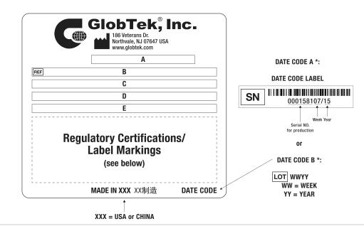
A=ICT / ITE / Medical Power Supply/Class 2/Household Power Supply B=P/N: (料号) TR9CC2000T00CFR6B C=Model (型号) GTM96180-1511-3.5-T3-CF D=Input (输入)100-240V~, 50-60 Hz, 0.6 A E=Output (输出)7.5 V == 2.0 A, 15.00W
