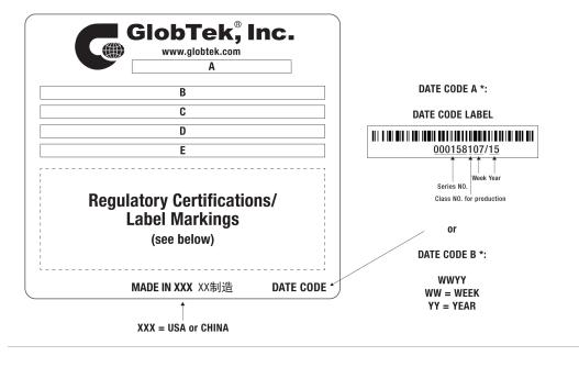
A=ICT/ITE Power Supply B=P/N: (料号) TR9CB3000CCP-N(R6B) C=Model (型号) GT-46200-1806-0.05-T3 D=Input (输入)100-240V~, 50-60 Hz, 0.5 A E=Output (输出)5.95 V === 3.0 A, 18.00W
