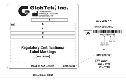
A=ICT / ITE / Medical Power Supply/Class 2/Household Power Supply B=P/N: (料号) TR9CA8000YL4CIM(R6B) C=Model (型号) GTM96600-4005-T3 D=Input (输入)100-240V~, 50-60Hz, 1.5A E=Output (输出)5.0 V ---- 8.0 A, 40.00W
