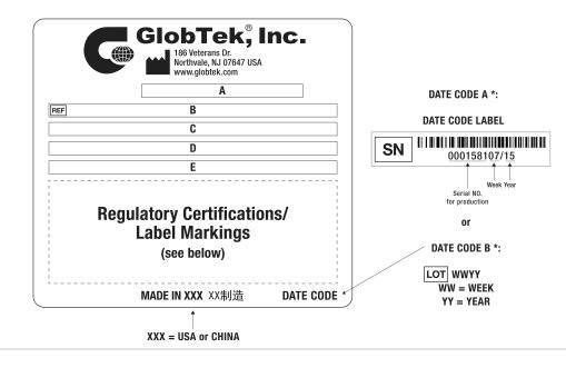
A=ICT / ITE / Medical Power Supply/Class 2/Household Power Supply B=P/N: (料号) TR9CA8000LCPIM(R6B) C=Model (型号) GTM96600-4005-T3 D=Input (输入)100-240V~, 50-60Hz, 1.5A E=Output (输出)5.0 V ---- 8.0 A, 40.00W
