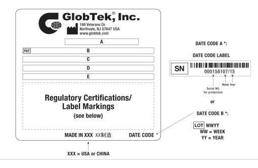
A=ICT / ITE / Medical Power Supply/Class 2/Household Power Supply B=P/N: (料号) TR9CA8000CCPIM(R6B) C=Model (型号) GTM96600-4005-T3 D=Input (输入)100-240V~, 50-60Hz, 1.5A E=Output (输出)5.0 V === 8.0 A, 40.00W
