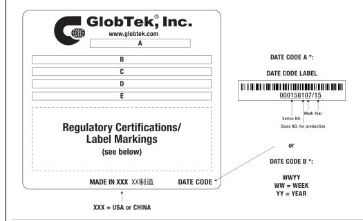
A=ICT / ITE / Medical Power Supply/Class 2/Household Power Supply B=P/N: (料号) TR9CA3000LCP-IM(R6B) C=Model (型号) GTM96180-1507-2.0-T3 D=Input (输入)100-240V~, 50-60 Hz, 0.6 A E=Output (输出)5.0 V == 3.0 A, 15.00W
