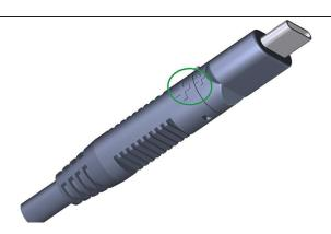
When installing T-USB-TYPE-C(R) changeable output Type C Plug, please match up the + Symbols on both the end of the output cord and the USB type C plug.
