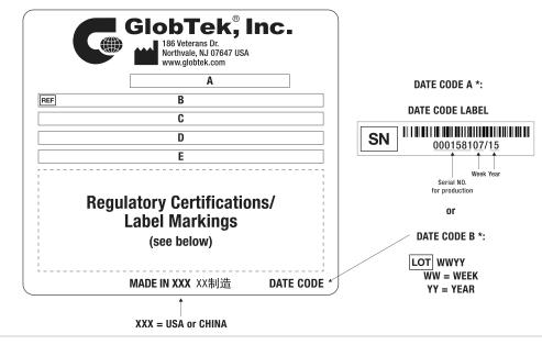
A=Medical/ICT/ITE/Household use Power Supply B=P/N: (料号) RR9LI1500LCPIMNAR6B C=Model (型号) GTM96300-3624-R3A D=Input (输入)100-240V~, 50-60 Hz, 1.0A E=Output (输出)24.0 V === 1.5 A, 36.00W
