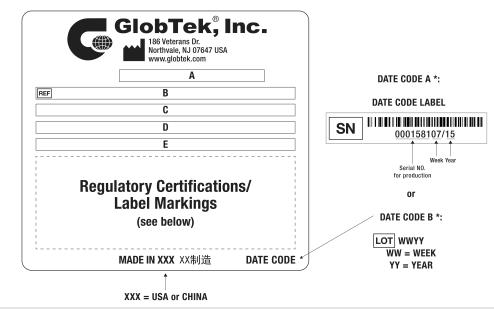
A=Medical/ICT/ITE/Household use Power Supply B=P/N: (料号) RR9LH2000T00NACIMR6B C=Model (型号) GTM96300-3619.5-1.5-R3A D=Input (输入)100-240V~, 50-60 Hz, 1.0A E=Output (输出)18.0 V === 2.0 A, 36.00W
