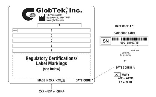
A=USB Power Delivery (PD) Source, ICT/ITE/Medical B=P/N: (料号) RR9KZ3000USBCRAR6B C=Model (型号) GTM96605-G2A1-R2-RA D=Input (输入)100-240V~, 50-60Hz, 1.5A
