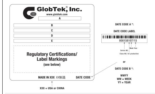
A=ICT / ITE / Medical Power Supply/Class 2/Household Power Supply B=P/N: (料号) RR9KX750T00-IMR6B C=Model (型号) GTM96300-3648-R2 D=Input (输入)100-240V~, 50-60 Hz, 1A E=Output (输出)48.0 V == 0.75 A, 36.00W
