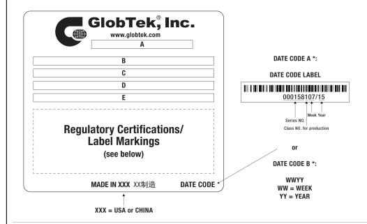
A=ICT / ITE / Medical Power Supply/Class 2/Household Power Supply B=P/N: (料号) RR9KI2700LCP-IMR6B C=Model (型号) GTM96600-6524-R2 D=Input (输入)100-240V~, 50-60 Hz, 1.5 A E=Output (输出)24.0 V == 2.7 A, 65.00W
