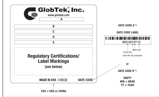
A=ICT / ITE / Medical Power Supply/Class 2/Household Power Supply B=P/N: (料号) RR9KI2500LRPCIMR6B C=Model (型号) GTM96600-6024-R2 D=Input (输入)100-240V~, 50-60 Hz, 1.5 A E=Output (输出)24.0 V == 2.5 A, 60.00W
