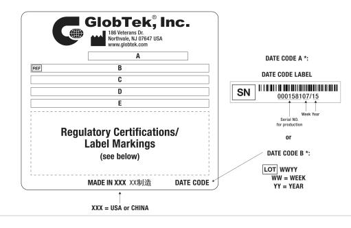
A=ICT / ITE / Medical Power Supply/Class 2/Household Power Supply B=P/N: (料号) RR9KI1500LCPIMNAR6B C=Model (型号) GTM96300-3624-R2 D=Input (输入)100-240V~, 50-60 Hz, 1A E=Output (输出)24.0 V === 1.5 A, 36.00W
