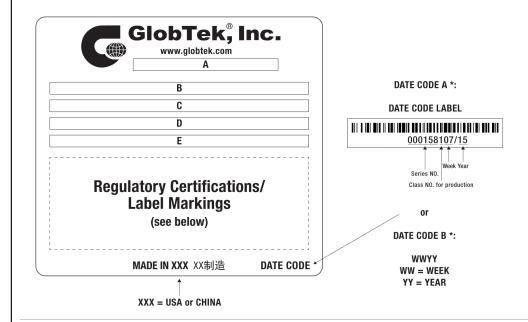
A=ICT / ITE / Medical Power Supply/Class 2/Household Power Supply B=P/N: (料号) RR9KI1500CCPIMNAR6B C=Model (型号) GTM96300-3624-R2 D=Input (输入)100-240V~, 50-60 Hz, 1A E=Output (输出)24.0 V === 1.5 A, 36.00W
