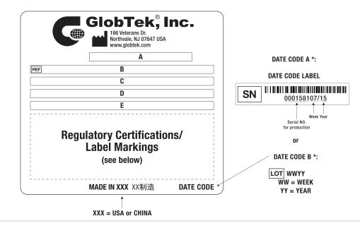
A=ICT / ITE / Medical Power Supply/Class 2/Household Power Supply B=P/N: (料号) RR9KE5410CCP-IMR6B C=Model (型号) GTM96600-6512-R2 D=Input (输入)100-240V~, 50-60 Hz, 1.5 A E=Output (输出)12.0 V === 5.41 A, 65.00W
